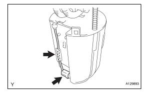
(b) Separate the connector and disengage the clamp.
