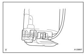
(b) Disengage the 5 claws and separate the fuel pump from the fuel pump case.
