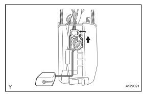
(b) Disengage the claw and remove the sender gauge by sliding it in the direction shown in the illustration.
