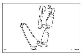
(c) Disconnect the connector from the fuel pump.
